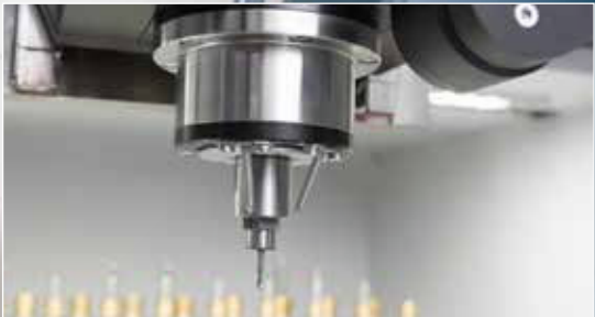
2 kW spindle and minimum-quantity coolant system
