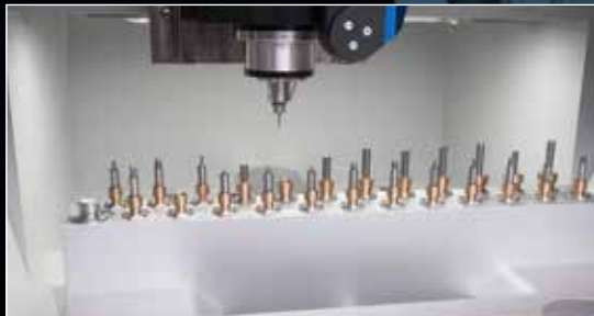
24-station tool magazine with integrated tool-length sensor
